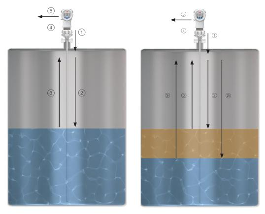
When two liquids are in the tank and are separated, if the dielectric constant difference between the two is more than 10, it is possible to detect the total level and the interface level at the same time. The radar wave will go through the first layer (having a low dielectric constant) and reach the top of the second layer (having a higher dielectric constant).
