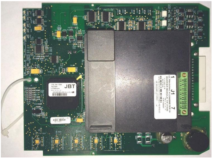
Figure 1-6: 3800 Series CPU Board with I.S. Barrier Board Piggy-Backed on CPU Board
