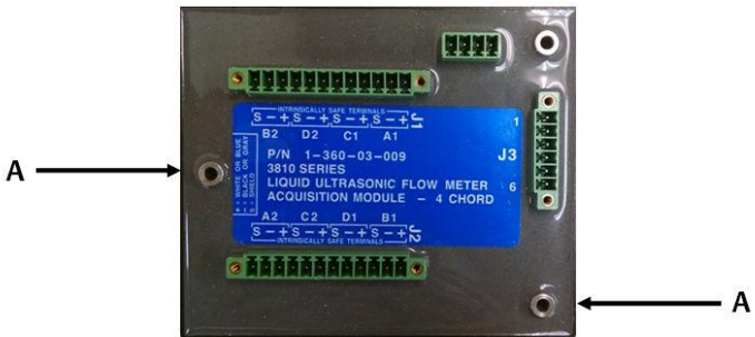
Figure 2-5: Acquisition Module Attachment Screws
