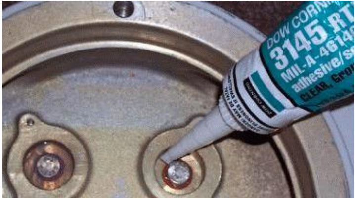
Figure 2-4: Apply RTV Sealant Around Bolts
