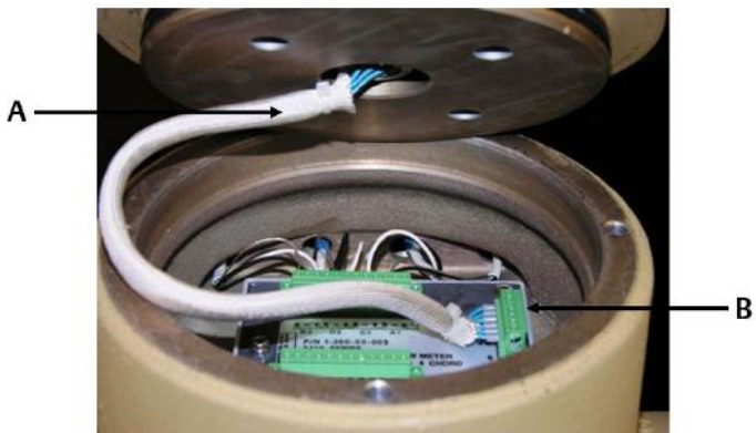
Figure 2-1: Remove Acquisition Cable and Module
