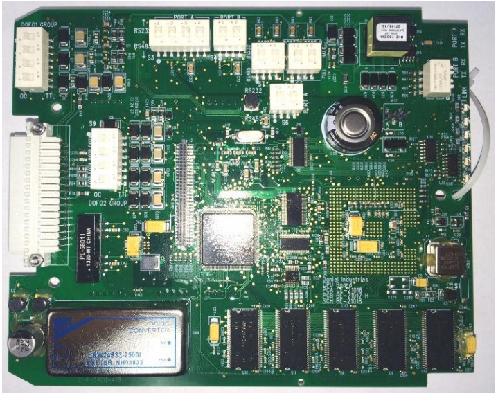
Figure 1-5: 3800 Series CPU Board Showing Switch Settings
