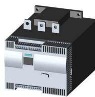
SIRIUS soft starter Values at 400 V, 40 °C standard: 203 A, 110 kW Inside-delta: 352 A, 200 kW 200-460 V AC, 230 V AC Screw terminals !!! Phased-out product !!! Successor is SIRIUS 3RW5, Preferred successor type is >>3RW5543-6HA14<<
