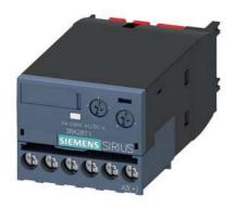
electronic timing relay, ON-delay, with semiconductor output, time range 0.05-100 s, 24-240 V AC/DC, 50/60 Hz, varistor for attenuation of the contactor coils integrated, screw terminal, can be snapped on at the front on contactors 3RT2.1 / 3RT2.2 and auxiliary contactors 3RH2
