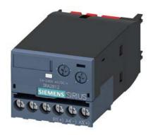
electronic timing relay, off delayed, with control signal and semiconductor output, time range 0.05-100 s, 24-240 V AC/DC, 50/60 Hz, varistor for attenuation of the contactor coils integrated, screw terminal, can be snapped on at the front on contactors 3RT2.1 / 3RT2.2 and auxiliary contactors 3RH2
