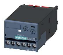
electronic timing relay, ON-delay, with semiconductor output, time range 0.05-100 s, 24-90 V AC/DC, 50/60 Hz, varistor for attenuation of the contactor coils integrated, screw terminal, can be snapped on at the front on contactors 3RT2.3/3RT2.4
