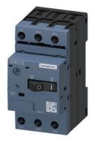
Circuit breaker size S00 for motor protection, CLASS 10 A-release 0.11...0.16 A N-release 2.1 A Screw terminal Standard switching capacity
