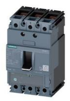
circuit breaker 3VA1 IEC frame 160 breaking capacity class N Icu=25kA @ 415V 3-pole, line protection TM220, ATFM, In=100A overload protection Ir=70A...100A short-circuit protection Ii=10 x In nut keeper kit
