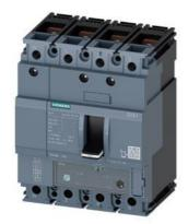
circuit breaker 3VA1 IEC frame 160 breaking capacity class N Icu=25kA @ 415V 4-pole, line protection TM240, ATAM, In=100A overload protection Ir=70A...100A short-circuit protection Ii=5...10 x In N conductor unprotected nut keeper kit
